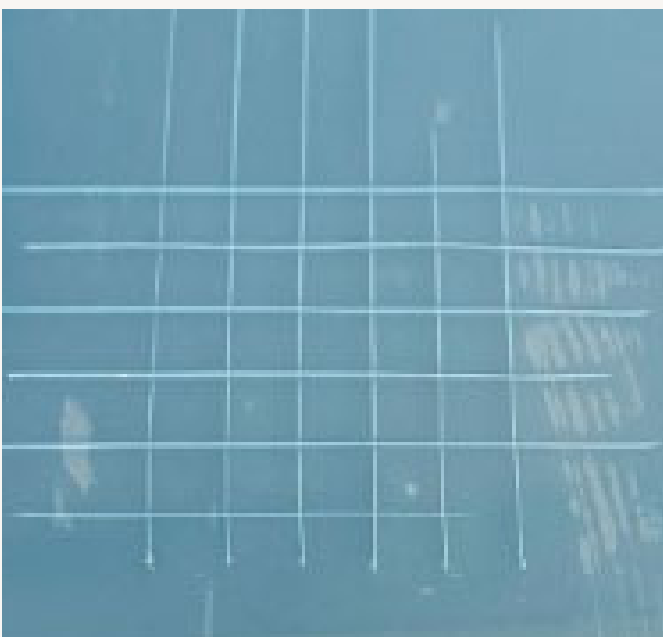
Cross-cut test (JIS K 5600-6), Grid spacing 3mm, Substrate LLDPE sheet
